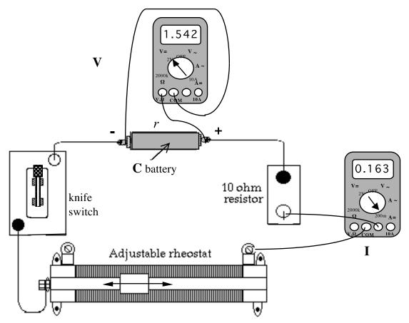
2.2. Make sure that the multimeter connected across the battery is set to the 2-Volt DC range (2 V=) and the one measuring current is set to the 200 mA DC range (A=). The multimeter connected across the battery should have wires connected to terminals labeled "COM" and "V". The multimeter measuring current should have wires connected to terminals labeled
