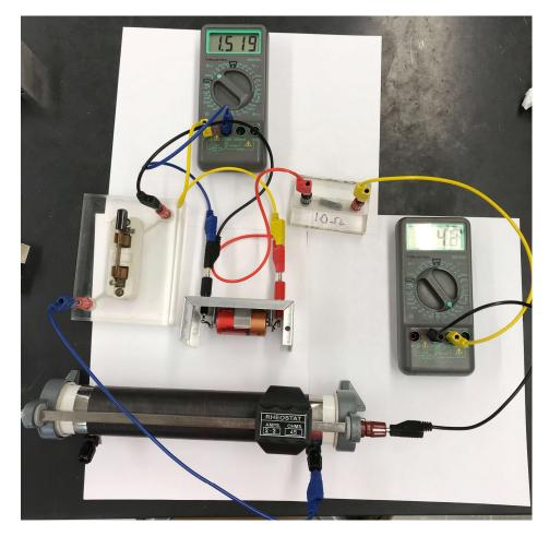
2.3. Create a voltage vs. current graph (voltage on the vertical axis and current on the horizontal axis) and attach the graph to your lab report. Calculate the straight line fit and find the slope and the y-intercept for that line. Find the internal resistance of the battery *r*.
