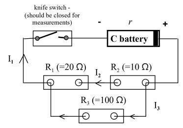
3.2. You will first measure the current that flows through the wire connecting R<sub>1</sub> and R<sub>2</sub>. That current, according to Kirchhoff's rules is equal to: I<sub>2</sub>. Insert the multimeter into the circuit as shown below.
