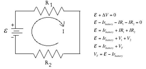
This process becomes more complicated if there is more than one loop present in the circuit. To find the currents in such a system, one needs to solve the set of equations made from the single loops. These equations may be determined from a process called the <u>loop method</u>:
