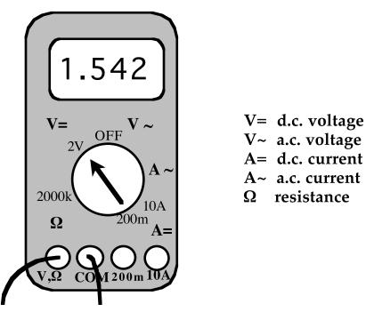
1.2. Connect the multimeter prongs to the tips of the battery holder (red tip to positive side of the battery and black tip to negative side of the battery). Record this voltage on your data sheet as the **emf** ( $\mathcal{E}$ ) of the battery.
